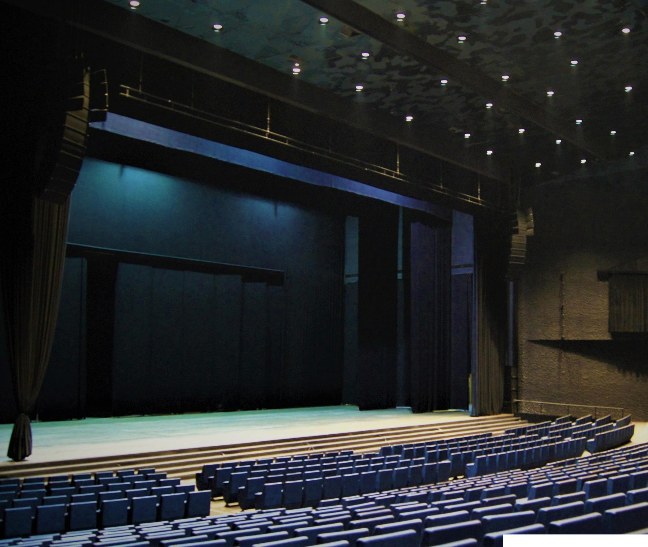
The stage is equipped with an American opening system with a **400 m<sup>2</sup>** black velvet Chopin curtain with a fixed non-programmable end of travel. It consists of two sections: 17 m wide and 14 m high.
